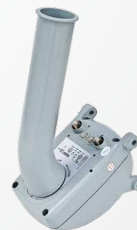
MH1 MOTOR 13/18V DC input F-Type Connector 1,2m Dish Max. 350mA Max. Current
