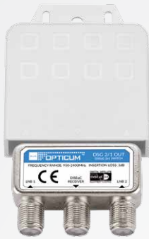
DSG2/1 OUT Frequency: 950-2400 MHz Insertion Loss: 3 dB Power: 12~20V DC/30mA
